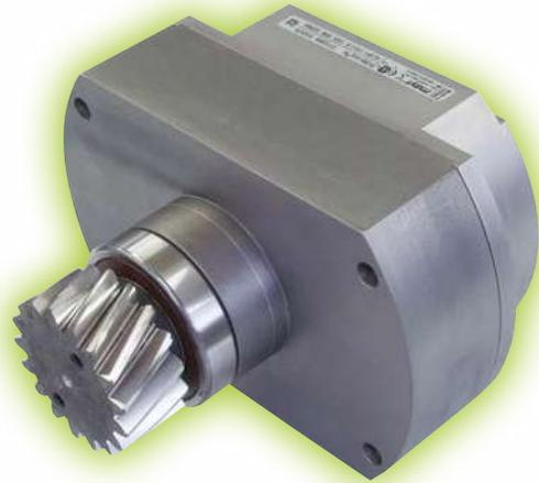
The ROBA®-pinionstop as an independent brake system engages directly and in any position onto the toothed rack and is closed in a de-energised condition. This safety brake is therefore able to offer high safety on power failure and EMERGENCY STOP as well as during installation and maintenance work.
