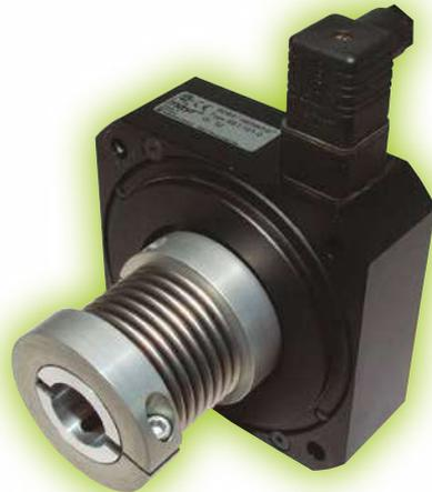
The ROBA<sup>®</sup>-alphastop<sup>®</sup> is a safety brake, installed between the servomotor and a bell housing. The brake toothed hub is combined with the smartflex<sup>®</sup> backlash-free steel bellows coupling. Frictionally-locking clamping rings ensure backlash-free torque transmission between the motor and the ball screw spindle.
