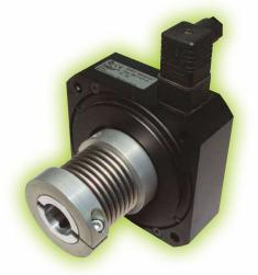
The ROBA®-alphastop® is a safety brake, installed between the servomotor and a bell housing. The brake toothed hub is combined with the smartflex® backlash-free steel bellows
